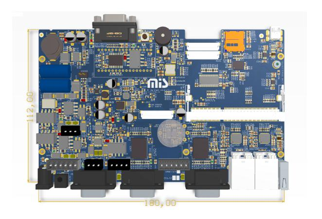
For a better mechanical stability the MIS-DIMM-AM437X SOM can be fasten to the TPANEL070X006 using the mechanical hole in the upper right corner.
